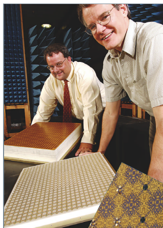
Researchers from the Georgia Tech Research Institute display a prototype antenna that replaces as many as five traditional antennas thanks to an innovative pattern of antenna elements (inset).
